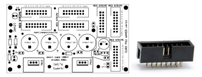
**2.** Once the connectors are installed, continue on and install the 4 diodes (be careful to match the stripes with the marking on the PCB), then the 4 small capacitors (unmarked, small rectangles), the two resistors (marked 1k) and the 2 LEDs (be careful to line up the flat edge of the LED with the marking on the PCB)
