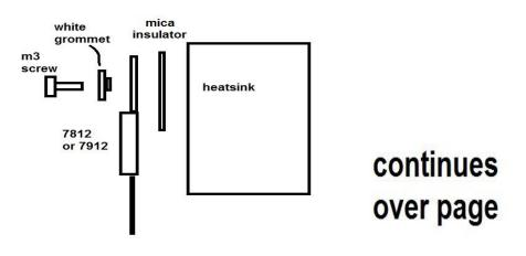
5. Once you have built the regulator/heatsink structures install them on the PCB, with the heatsink on the outside.
