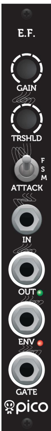
SET THE THRESHOLD OF THE GATE EXTRACTOR CIRCUIT. IT IS A VOLTAGE ABOVE WHICH THE AUDIO SIGNAL WILL TRIGGER THE GATE – SEE THE DIAGRAM BELOW! PLEASE NOTE, THAT, DEPENDING ON THE THRESHOLD SETTING, A SAME WAVEFORM CAN OUTPUT VARIOUS GATES
