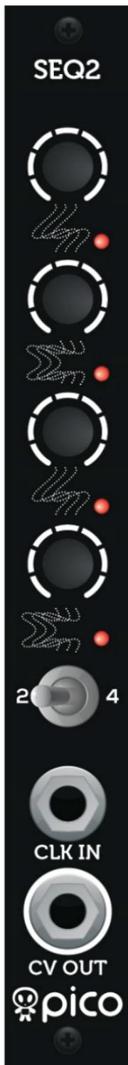
PATCH THE CLOCK OR AUDIO SIGNAL HERE. DUE TO LIMITED PANEL SPACE AND FUNCTIONALITY, PICO SEQ2 DOES NOT HAVE A GATE OUTPUT. WE RECOMMEND YOU TO USE STACKABLE PATCHCABLES TO COPY CLOCK SIGNAL TO ENVELOPE GENERATORS OR GET GATES FROM PICO TRIGGER OR LOGIC MODULES
